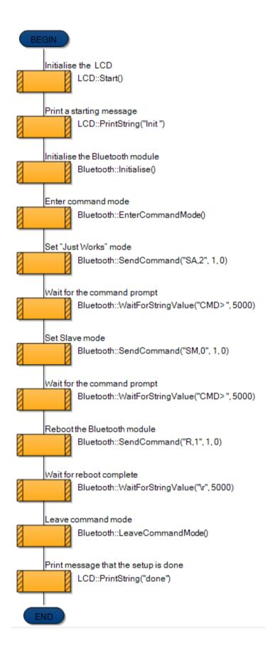
The SendCommand and WaitForStringValue macros, detailed previously, are used to setup the Bluetooth module as in the example shown here.
