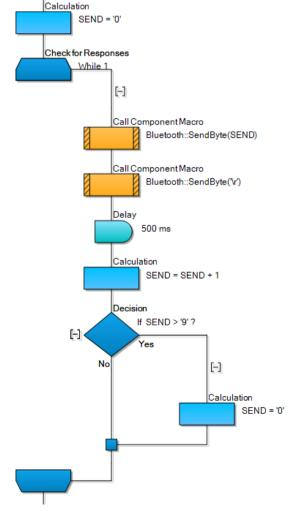
To demonstrate the connection is working a simple 0-9 repeating signal can be sent to be displayed on the receiving device.
