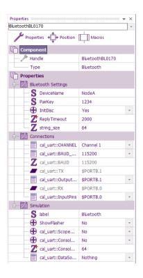
The Bluetooth BL0170 component is based on the RN4677 device and has a number of properties and connections that can be set by the user.
