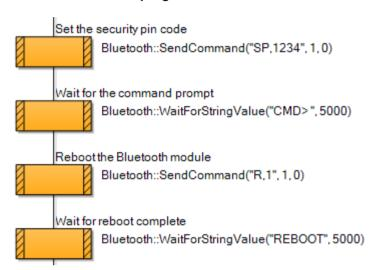
Pairing is a key process in Bluetooth operations. The passkey needs to be configured, and as with all "set" commands, is actioned after a device reboot, which can be done with the "R,1" command.
