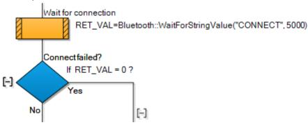
Once a command has been sent the WaitForStringValue can be used to check that the expected reply was received.
